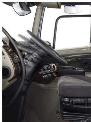
The low cab floor eases frequently getting in and out, while the flat-topped engine tunnel still enables good cross-cab access.
