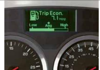
Kenworth's Multi-function Highline Display provides the driver with important real-time information on truck performance. The touch of a button displays up-to-the-second readouts on cumulative trip fuel economy, optimum RPM for maximizing fuel efficiency, and system diagnostics (in language a lay person can understand). Comprehensive truck specification data – unique to the vehicle – is also available to speed troubleshooting and parts replacement.
