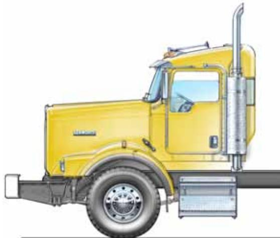
Perfect for snowplows, municipal dump trucks, mixers, refuse trucks and crane trucks that require front engine power take-off (FEPTO). The Kenworth factory-installed FEPTO avoids aftermarket retrofit problems. The 1,440-sq. in. radiator includes a modified bottom tank for PTO shaft clearance. A front-frame extension provides space for front-mounted equipment like hydraulic rams or hose reels.
