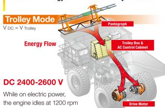
directing power only to the auxiliaries and the hydraulic pump - even when the machine is being driven uphill under load.
