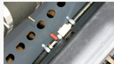
Fuel tank water drainage cock
