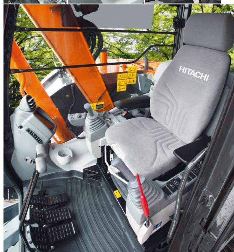
Shown equipped with air suspension seat, attachment pedal, sun visor and blade leve
