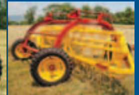
Offset wheels are set close to the basket, so the tines closely follow the ground for cleaner raking and more hay.
