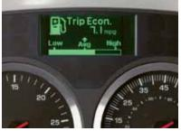
Kenworth's Multi-function Highline Display provides the driver with important real-time information on truck performance. The touch of a button displays up-to-the-second readouts on cumulative trip fuel economy, optimum RPM for maximizing fuel efficiency, and system diagnostics (in language a lay person can understand). Comprehensive truck specification data – unique to the vehicle – is also available to speed troubleshooting and parts replacement.
