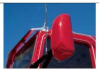
Your T800 can be outfitted with heated, motorized aerodynamic mirrors to add style, while the foldaway design resists damage if struck.
