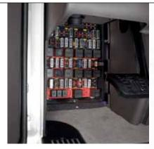
The T800's power distribution box puts all circuit protection elements – fuses, relays and breakers – in one quick-to-reach location.
