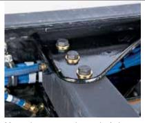
Heavy-duty crossmembers and 3-hole gussets strengthen a T800's backbone, preparing it for the pounding your job dishes out. They can be replaced in less than 10 minutes with no special tools.
