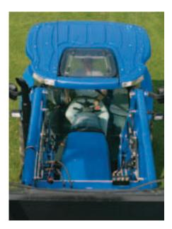
The Horizon<sup>™</sup> cab features an optional high-visibility roof panel for an easy view to a raised loader bucket.
