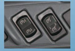
Push buttons for constant rpm and cruise control.
