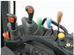
AutoShift™ transmissions provide automatic shifting in the field or one the road. You program the shift point and shuttle preferences.
