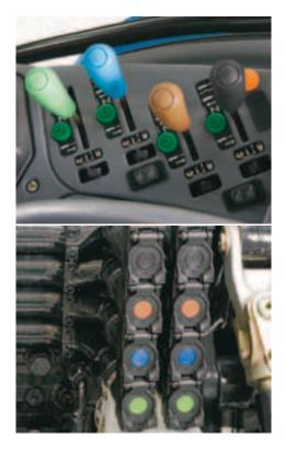
Hydraulic control levers and remote coupler dust covers are color-coded to assist with easy implement hook up and control.
