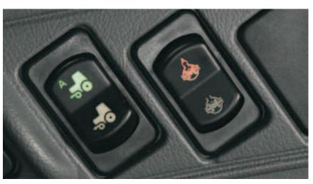
The Terralock™ system automatically controls FWD and differential lock engagement to give you maximum traction and control.
